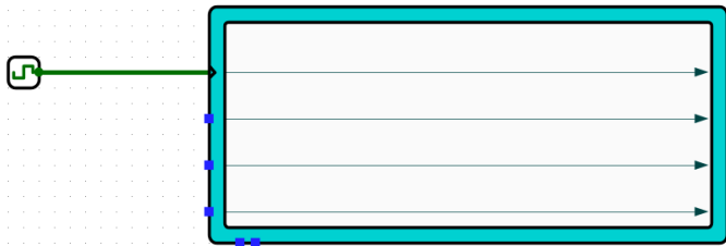
FIGURE 1. Odd Number of Inverters Will Always Oscillate
