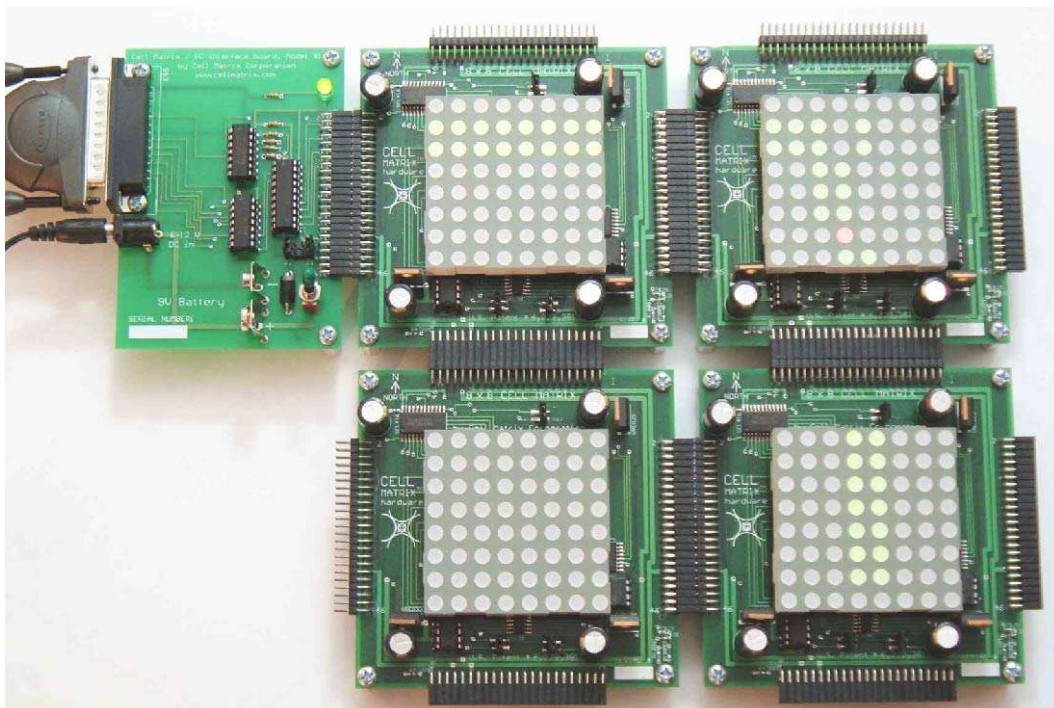
FIGURE 5 - PC INTERFACE BOARD CONNECTED TO FOUR CELL MATRIX MOD 88 BOARDS This implements a 16x16 Cell Matrix
